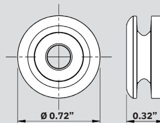
**Material:** ABS (Fix) & Nylon PA6, 30% glass filled (Button)
