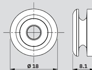
**Material:** Nylon PA6, 30% glass filled (Button & Fix)
