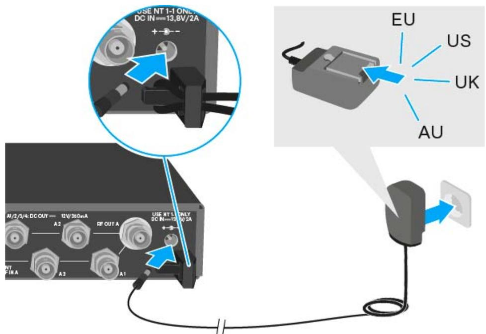
To completely disconnect the ASA 214 antenna splitter from the power supply system:
