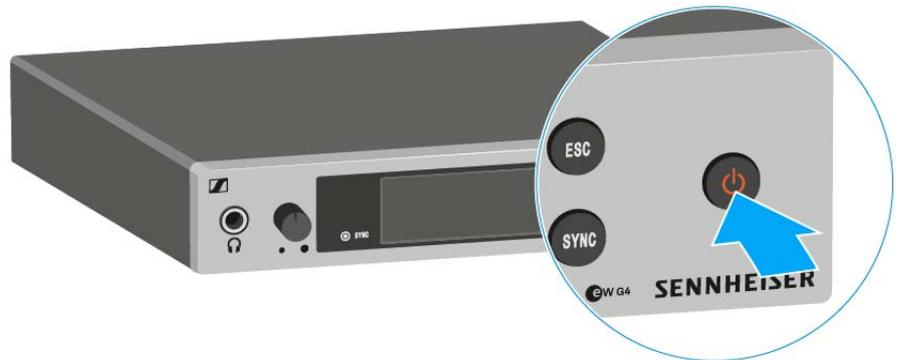
To switch the receiver to **standby mode**:
