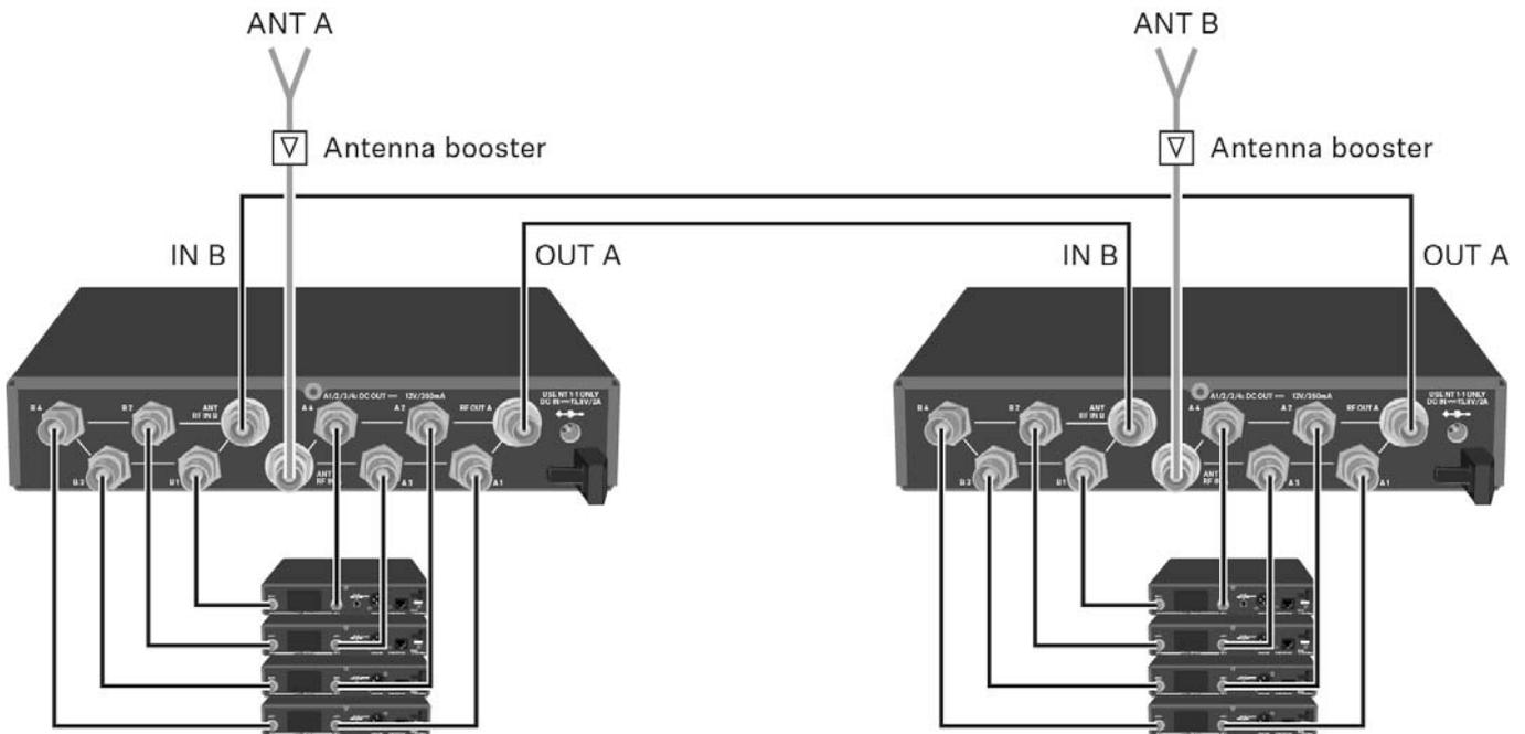
Option 3: Two antennas supply a 8-channel system
