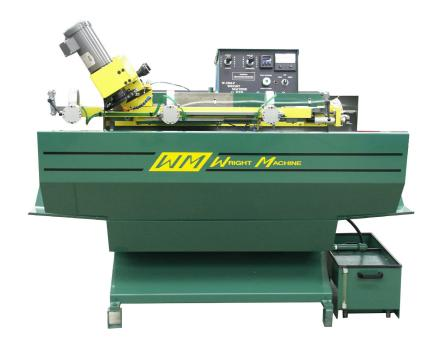
The W-1902-P Quad quickly and accurately sharpens the sides of swaged or stellite® tipped bandsaws. The periphery grind option gives the operator an efficient and highly accurate finish grind, increasing saw performance. The "for bandsaws only" design allows features that improve accuracy and speed.
