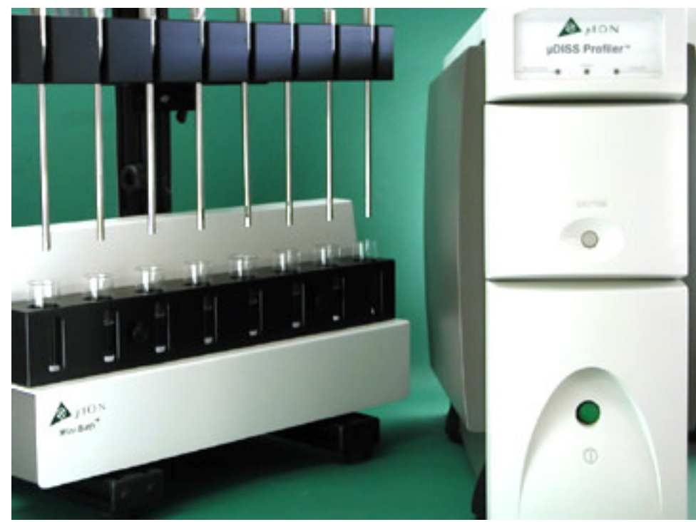
Figure 2. µDISS Profiler from pION INC uses a temperature controlled Mini-Bath and 8 integrated diode array spectrometers to collect full UV spectra as often as once per one second.
