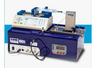
The Surface Dissolution Imager (SDI) is an instrument marketed by Sirius Analytical. It uses ultra-violet light to monitor the dissolution of active pharmaceutical ingredients (APIs) at the surface. It has been used to study the dissolution behavior of APIs, co-crystals, salts, solid dispersions and stents.
