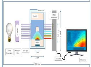
The flow cell was adapted so that the surface of a full dosage form could be analyzed. This resulted in a path length of 25 mm for the UV light; therefore improving the limit of detection of the API. To distinguish between dissolved and undissolved material two wavelegths were used: visible (550 nm) and UV (254 nm). It is proposed that any dissolved material would only be detected by the UV wavelength, undissolved would be observed using both wavelengths.
