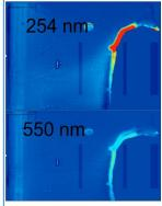
The white circles highlight areas of higher absorbance flowing away from the tablet surface, this is most likely due to dissolved diclofenac as there was no significant evidence of it at 550 nm.
