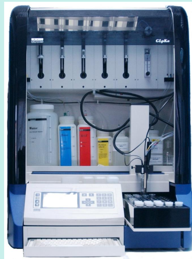
pK a measurements in 2-propanol were made using Sirius GLpKa (above). During the titrations the measurement cell was purged with an inert gas atmosphere. Probes and samples were moved under full automation to minimise user exposure to 2-propanol.
