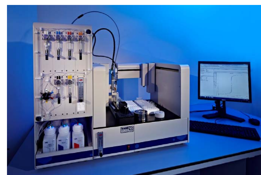
Fig. 2 – SiriusT3 automated platform for pK a determination through Fast-UV analysis.
