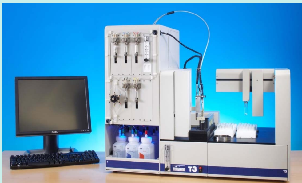
Fig. 1: Sirius T3 automated platform for measuring pKa, logP, solubility and dissolution properties.
