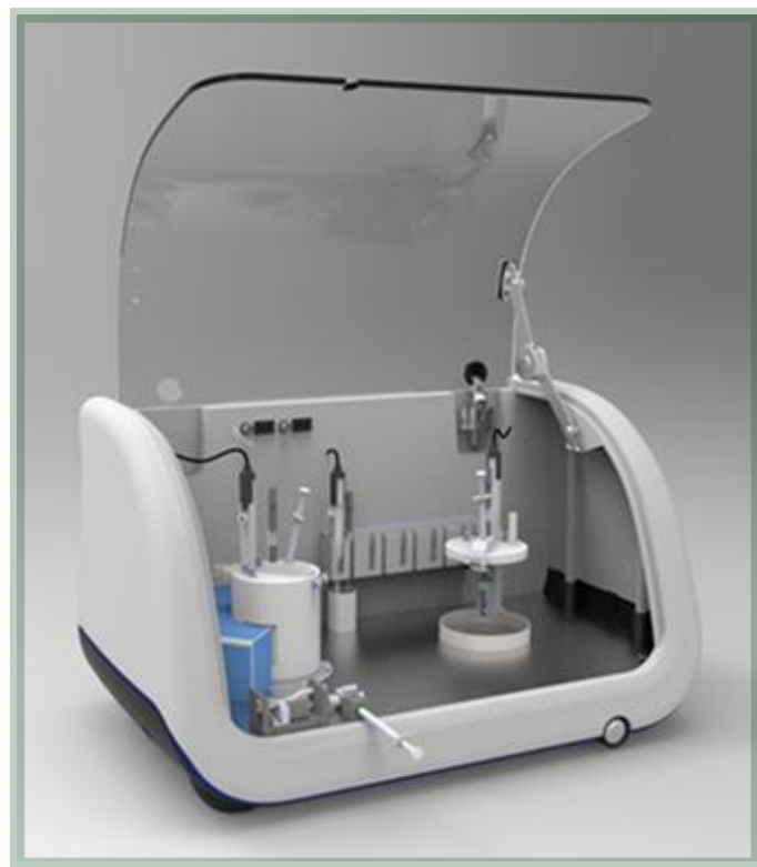
Fig. 2 Pion Scissor, a novel instrument for in vitro testing of biopharmaceutical formulations
