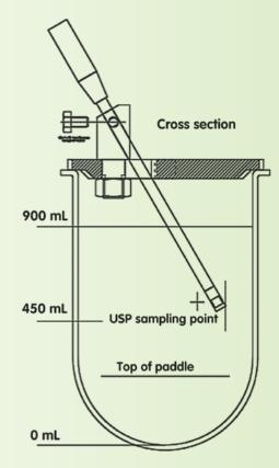
By angling the fiber optic probe at 30° into the dissolution vessel you accomplish the following:
