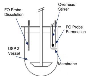
Figure 3. Schematic of Dissolution - Flux device used in this study.
