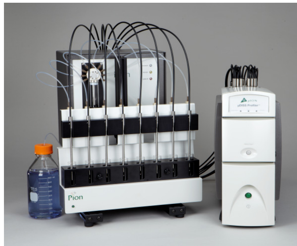
Figure 2. The \mu DISS Profiler monitors concentration in real time with ability to dynamically change media in 8 temperature controlled vessels using only 1 – 20 mL volume.
