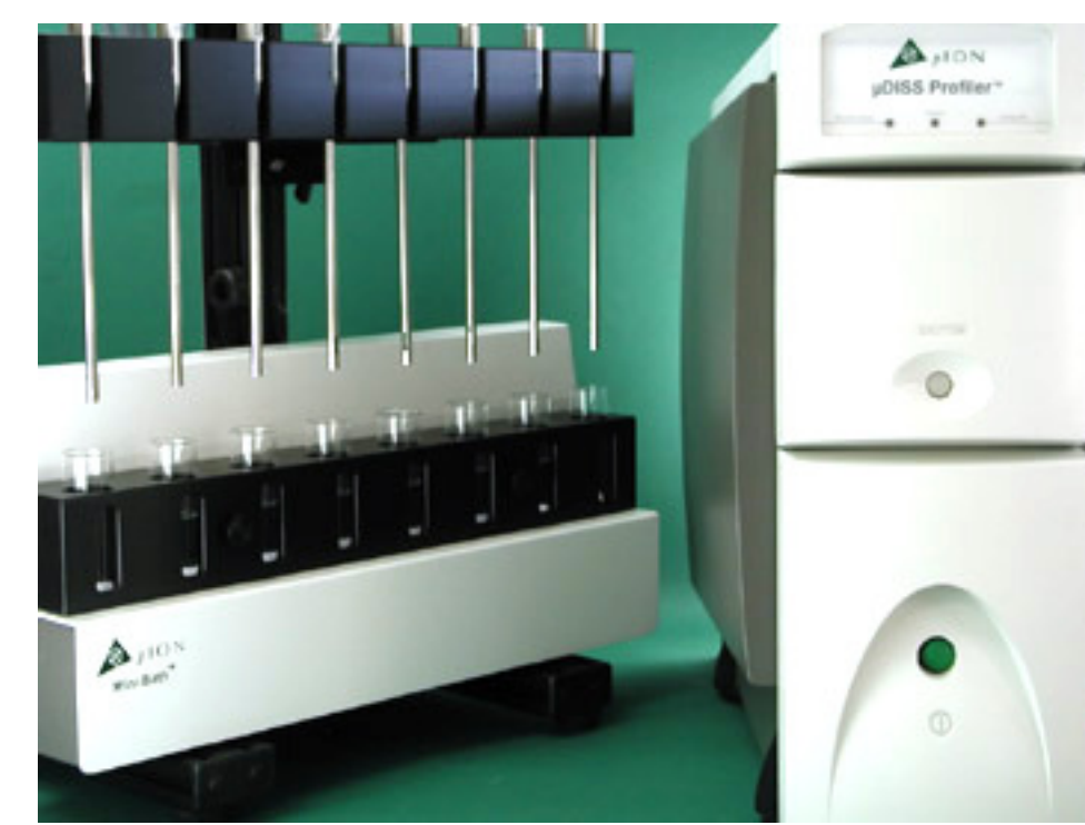
Fig. 1. µDISS Profiler PLUS TM from pION INC uses a temperature controlled Mini-Bath and 8 integrated diode array spectrometers to collect full UV spectra as often as once per one second.
