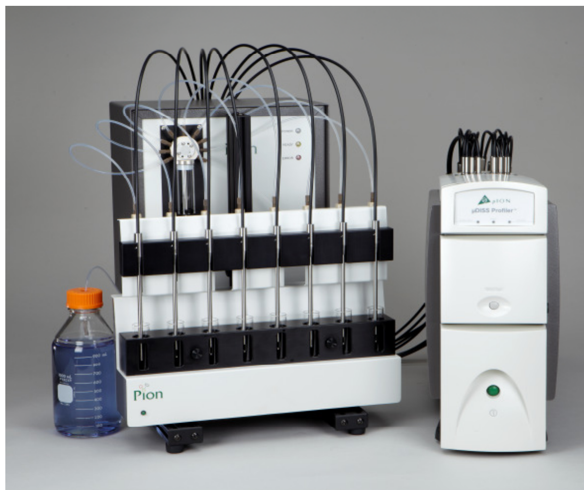
Figure 2. The μDISS Profiler monitors concentration in real time with ability to dynamically change media in 8 temperature controlled vessels using only 1 – 20 mL.
