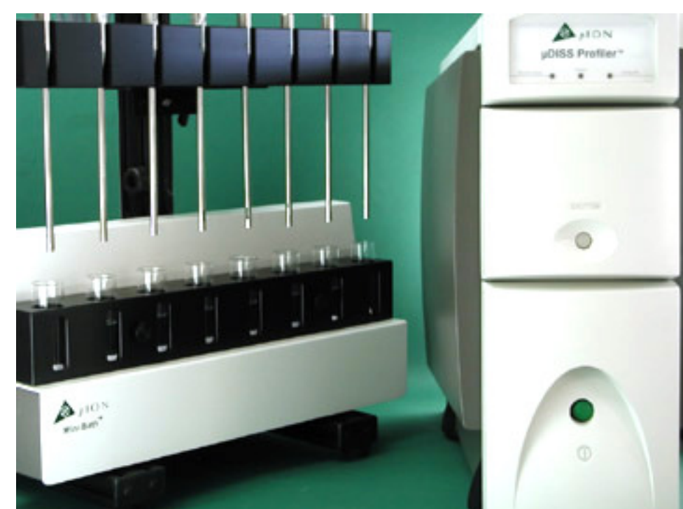
Figure 2. The \mu DISS Profiler from Pion Inc monitors concentration in real time in 8 temperature controlled channels using only 1 – 20 mL of dissolution media.
