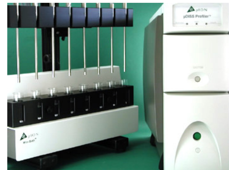
Figure 2. The \mu DISS Profiler from Pion Inc monitors concentration in real time in 8 temperature controlled vessels using only 1 – 20 mL of dissolution media.
