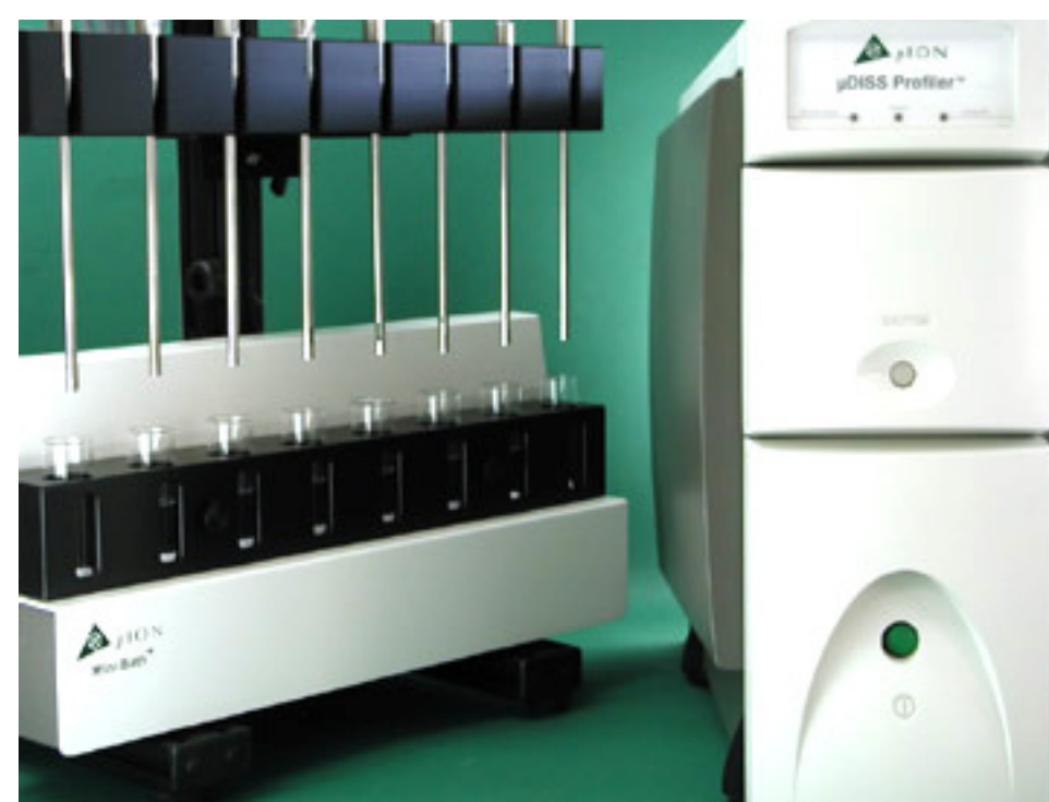
Figure 2. The \mu DISS Profiler from Pion Inc. monitors concentration in real time in 8 temperature controlled vessels using only 1 – 20 mL of dissolution media.
