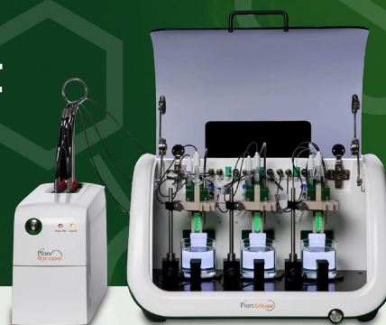
The Pion SCISSOR N3 (right) and Rainbow R6 (left) set up to monitor in situ release of a formulation.
