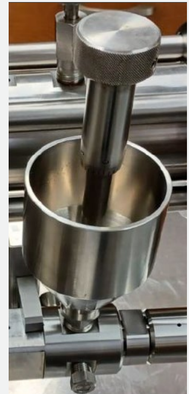
Some models allow for certain powders to be incorporated directly into the mixing stream.
