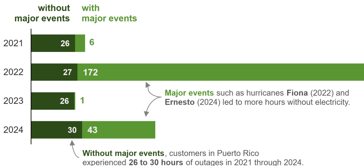
Figure 1: Average duration of annual electricity interruptions in Puerto Rico starting in 2021. (Source: U.S. Energy Information Administration) 7
