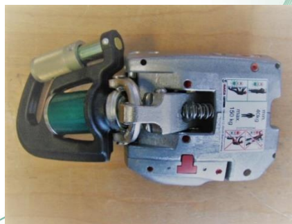
Fig. 1-2: Guided-type fall arrester types 0529.74 and 0529.7430
