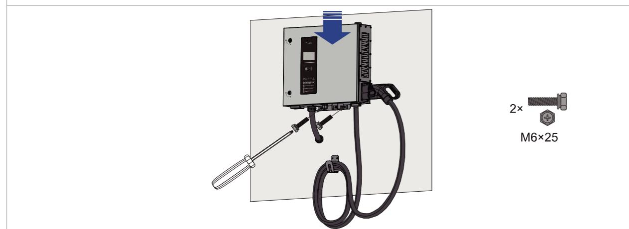
2) Place charger onto bracket. Align the back chassis of the charger with the corresponding slot on the bracket. Slowly slide down the charger until it sits firmly on the bracket. Fasten two screws from the bottom.
