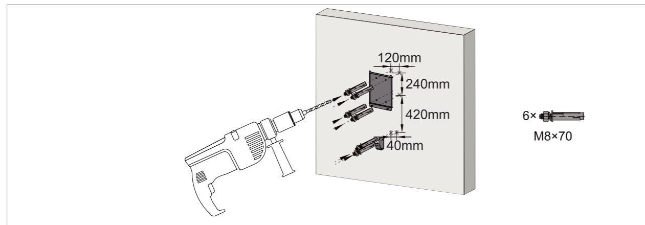
1) Use the bracket and hook to mark drill holes. Mount bracket and hook onto the wall. Use the expansion bolts in the accessory kit or choose proper mounting screws for different types of wall. A drilling machine might be needed for certain conditions.
