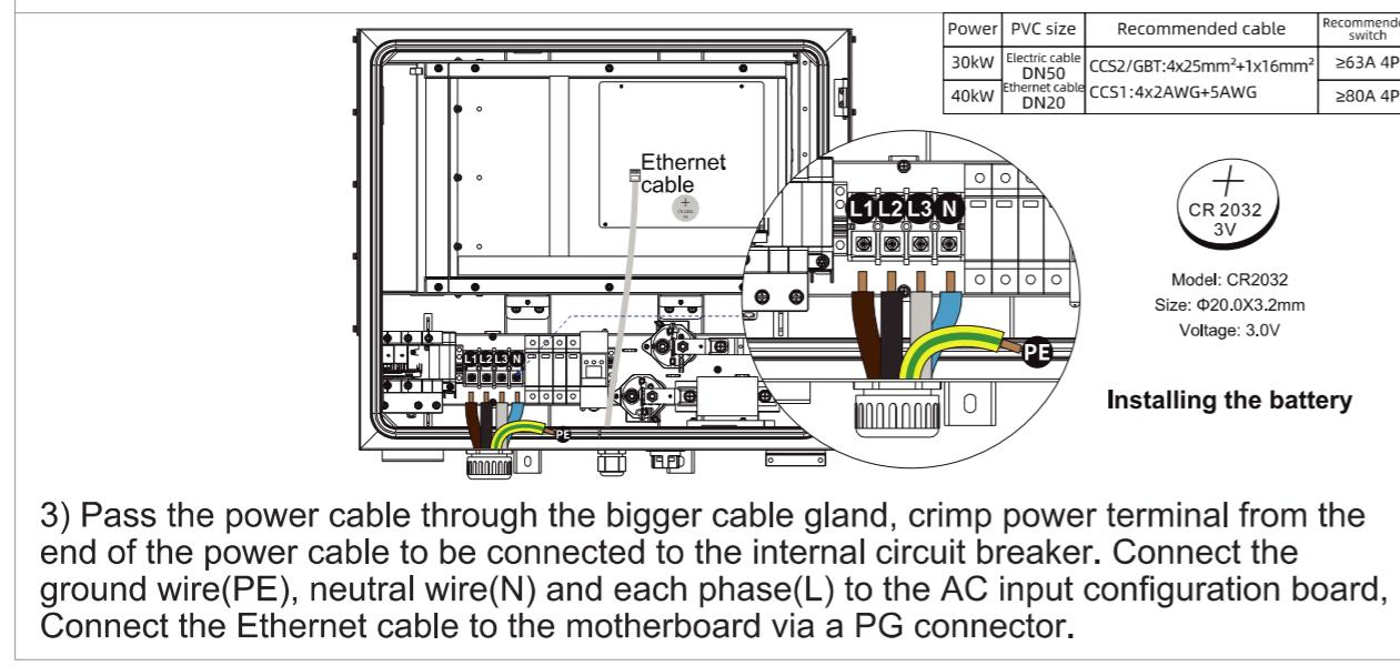
3) Pass the power cable through the bigger cable gland, crimp power terminal from the end of the power cable to be connected to the internal circuit breaker. Connect the ground wire(PE), neutral wire(N) and each phase(L) to the AC input configuration board. Connect the Ethernet cable to the motherboard via a PG connector.
