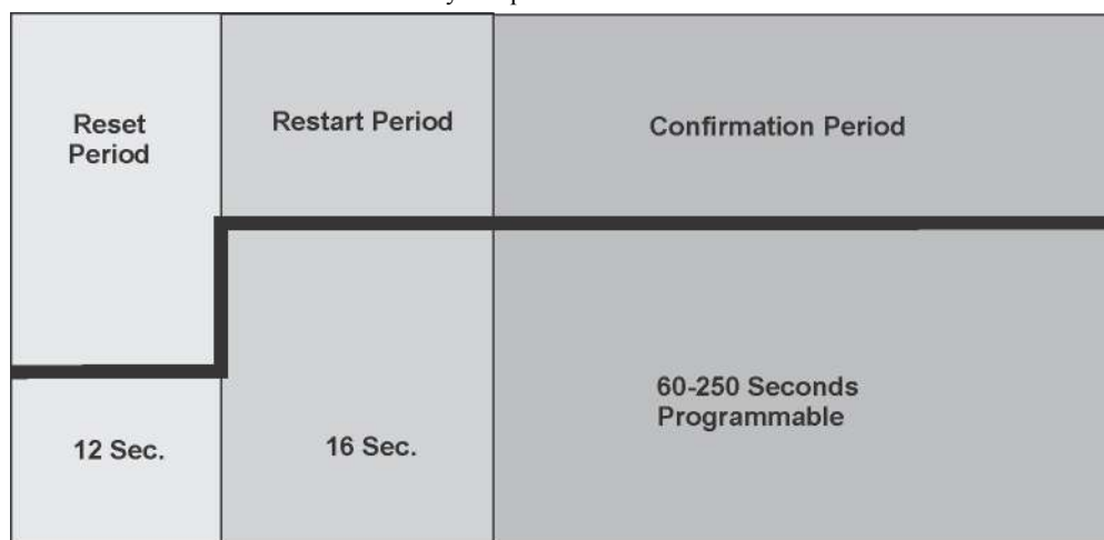
Figure 10.7 Smoke Verification Cycle
