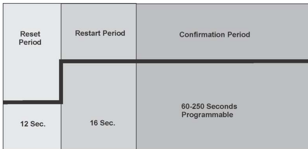
Figure 10.7 Smoke Verification Cycle
