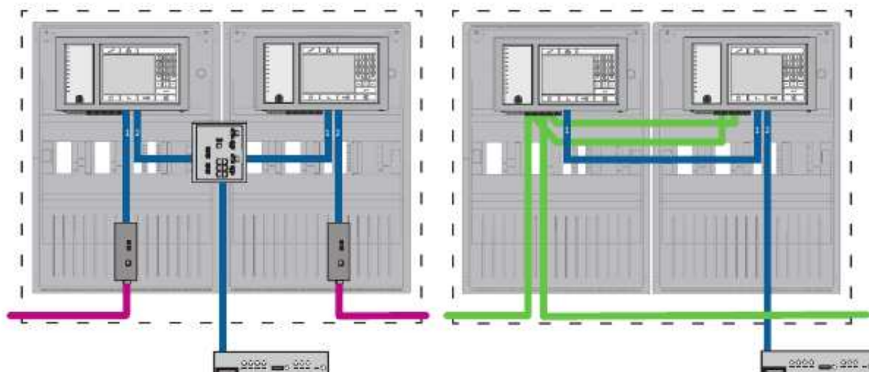
Figure 7.10: Left side: in Ethernet network Right side: in CAN network
