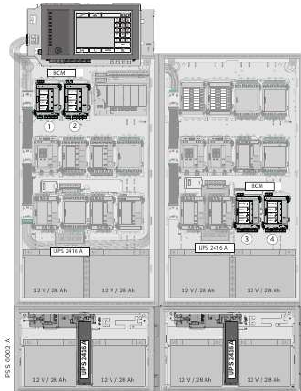
Figure 3.7: Configuration of 1 to 4 BCM modules (wall mounting)
