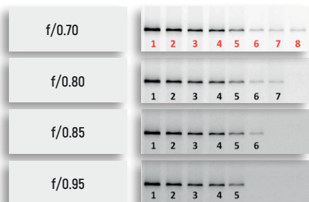
Figure 2. The HSR technology provides a better sensitivity by reducing the noise ground level. By keeping the background to its lowest floor level, the very faint signal can easily be detected and quantified.
