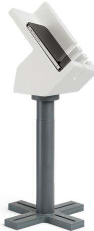
The Low Loss Mobile Holder is made of a special material with very low loss tangent ( $<0.0002$ ) and a dielectric constant close to air (1.075). These properties minimize the measurement impact of the holder. The holder also makes it very easy to move the phone or other small wireless devices in and out of the chamber and place the device in a repeatable position. Cable outlets are provided in strategic positions.
