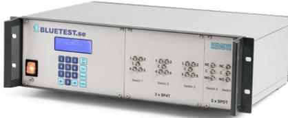
The ISS11 Instrument Switch makes it possible for the user to create a permanent test set-up around the RTS. All the instruments like network analyzers and communication testers can be connected to the chamber without time consuming re-cabling. ISS11 Instrument Switch contains three high performance SP4T switches and two optional SPDT switches for support of RTS with 4x4 MIMO. The switch is controlled via Ethernet and is fully integrated in the Bluetest Flow platform.
