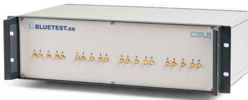
Even with 16 available measurement ports on the RTS there may be configurations where the measurement ports simply are not enough. The Combiner/Splitter units are the solution to this problem and come in two versions. CSU1 contains 4 pcs of 4-to-1 combiner/splitters and CSU2 contains 4 pcs of 2-to-1 combiner/splitters. Both units are 19" rack mountable and 3HU high.
