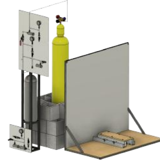
Figure 30: The full ethanol propellant tower test stand, with a linear rail system for housing the engine.
