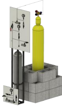
Figure 29: The ethanol propellant tower test stand. The cinder block assembly and K-bottle are also shown.
