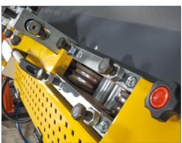
Straightening wheels are produced by most quality material with heat treated. It makes the machine firstly then parts very agile.
