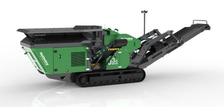
The versatile, mobile J3C crusher moves nimbly around in small spaces, and continues moving while crushing.
