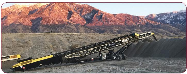
With our patented track technology, Masaba's Magnum Telescoping Conveyor is the safest, most rugged telescoping conveyor on the market. The patented track design provides constant positive traction and smoother operation of the stinger, improving long term durability with minimal annual maintenance required. Ranging from 130' - 190', we have a Magnum to suit your needs.
