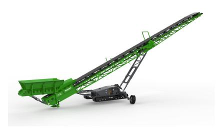
The design allows for the wheels to be fully folded for transport, delivering true site-tosite portability. The ST80TF features a large capacity hopper (5.75 cu.m. or 7.5 cu. yd.) with adjustable height, ensuring optimized operational efficiency on the job.
