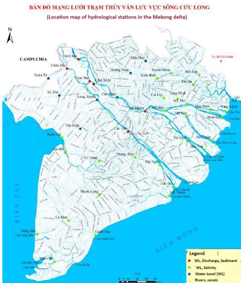
Figure 16: Location map of hydrological stations in the Mekong delta for model calibration
