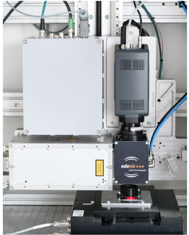
Figure 4: INSIGHT-L inspection head with active pilot laser
