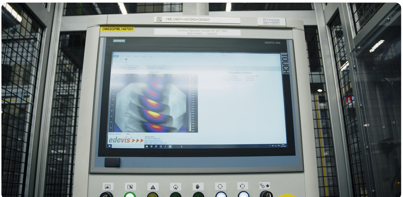
Fig. 4 Live display of the thermographic results
