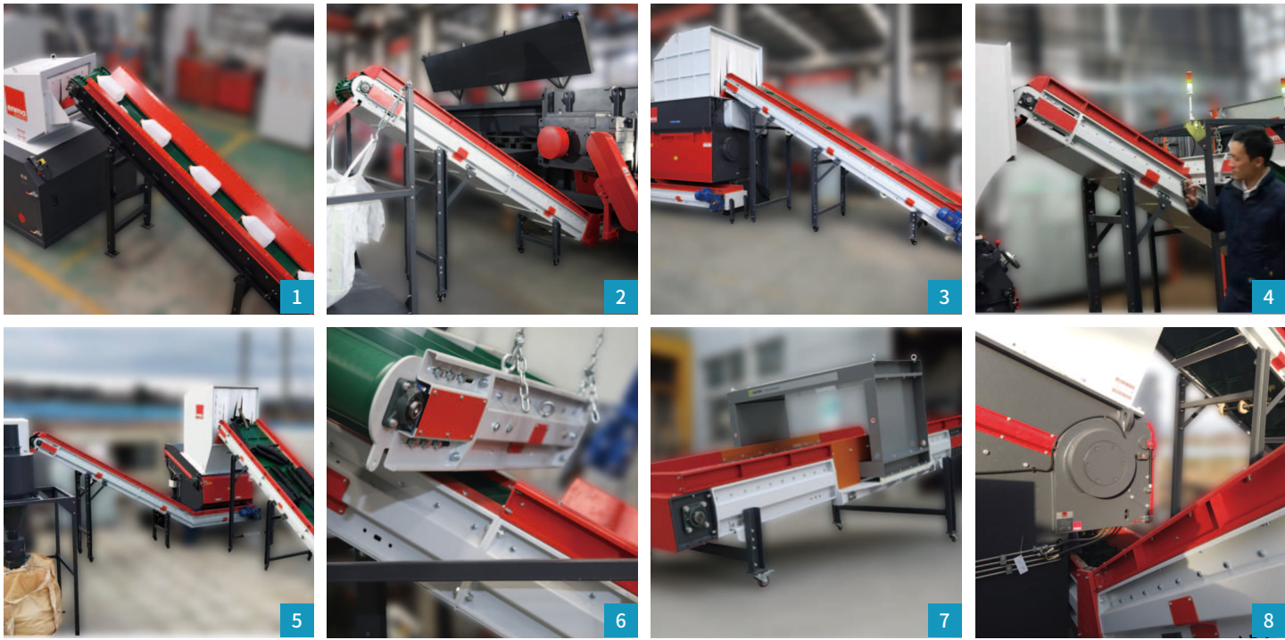
1.Recycling within plant 2.Pipe Recycling and Outputting 3.Inputting & Outputting 4.Conveyor for electronic wire recycling 5.Shredder inputting & outputting 6.Belt type metal separator 7.Feeding conveyor & metal detector 8.Shredder outputting conveyor
