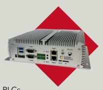
The Eureka Controller seamlessly connects to robots, cameras, sensors, and PLCs, orchestrates them in powerful Robotics & Al applications.
