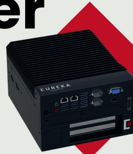
The Eureka Controller seamlessly connects to robots, cameras, sensors, and PLCs, and orchestrates them for powerful Robotics & AI applications. Built-in GPU enables fast, on-device vision processing.
