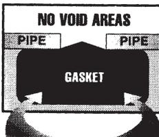
With no void areas in gasket there is no place for contamination to hide. A quick disassembly and visual inspection is all that is necessary.
