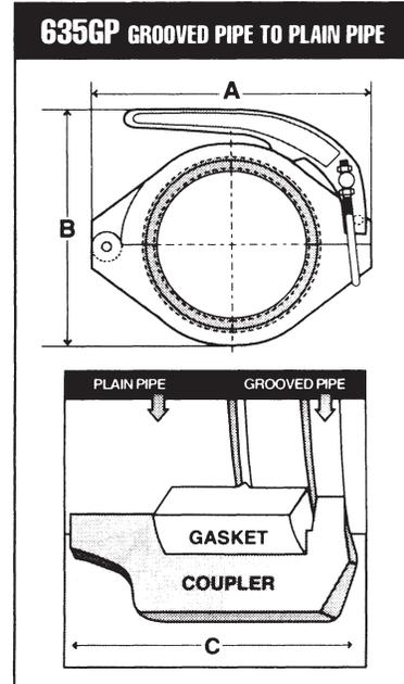
The aluminum quick couplers are furnished in different styles. The grooved pipe to grooved pipe coupler part numbers are 632GG, 634GG, 635GG, and 639GG. These couplers are superior to other couplers on the market today for the transportation industry. They are completely manufactured out of 713 aluminum and stainless steel for light weight and have SAE 841 oil impregnated bronze bushings in all pivot points. The couplers are corrosion resistant, they are adjustable, and are also easy to operate.
