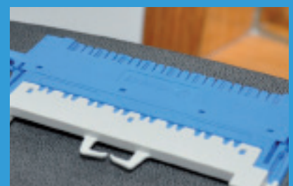
A connector for Toyota made of PBT with 30% GF. This part runs on a VE 600.
