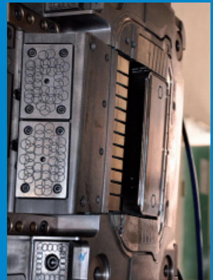
Mold test with the MCF-Technology on a Jupiter 3,300 tons.
