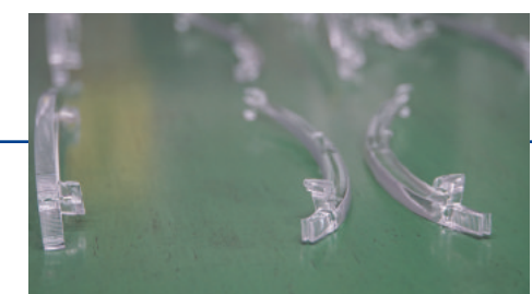
LightGuide STI with 60 g. shot weight of PMMA, manufactured on a Zhafir Venus II machine with 2 + 2 cavities and 65 second cycle time.
