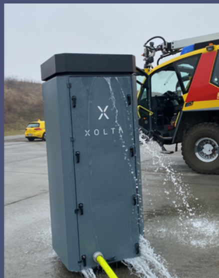
Figure 7 – Water filling tests has been performed to ensure sufficient design of the cabinet and sealings. The racks were required to be filled with water within 10 minutes, and the 2nd test was successful.
