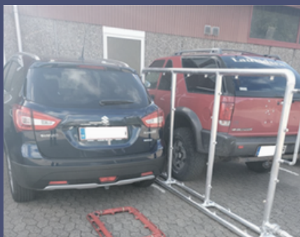
Figure 3 – Specialised sprinkler rack to cool burning EV and avoid spreading.
