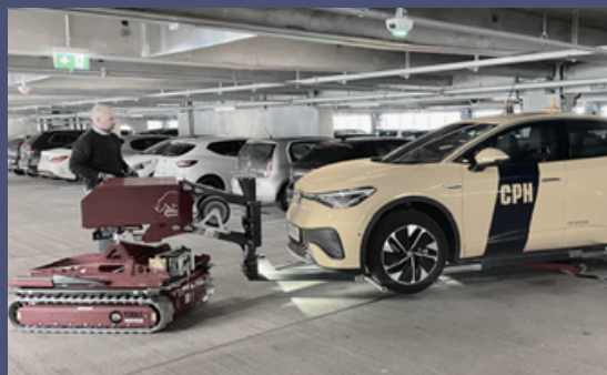
Figure 4 – FirstMover-tool used to move EVs in case of fire.
