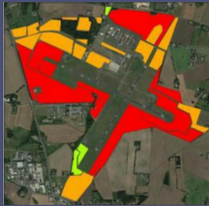
Figure 4 – Visualisation of potential areas for PVs without antireflective coating at CPH. These maps are part of a screening phase and do not show the actual applicability of the areas within the airport. Green: feasible area, Orange: possible area, Red: not possible.
