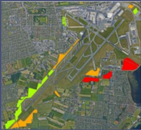
Figure 4 – Visualisation of potential areas for PVs without antireflective coating at CPH. These maps are part of a screening phase and do not show the actual applicability of the areas within the airport. Green: feasible area, Orange: possible area, Red: not possible.
