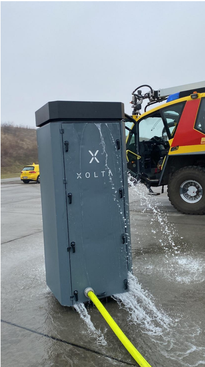
Figure 25 – Water filling tests has been performed to ensure sufficient design of the cabinet and sealings. The racks were required to be filled with water within 10 minutes, and the 2nd test was successful.
