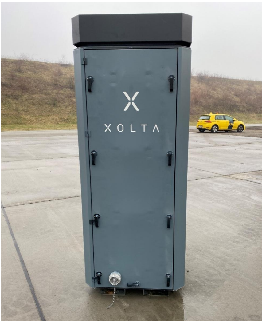
Figure 24 – Individual battery rack from Xolta. All racks are equipped with a connector for a fire hose, so they can be filled with water in case of fire.
