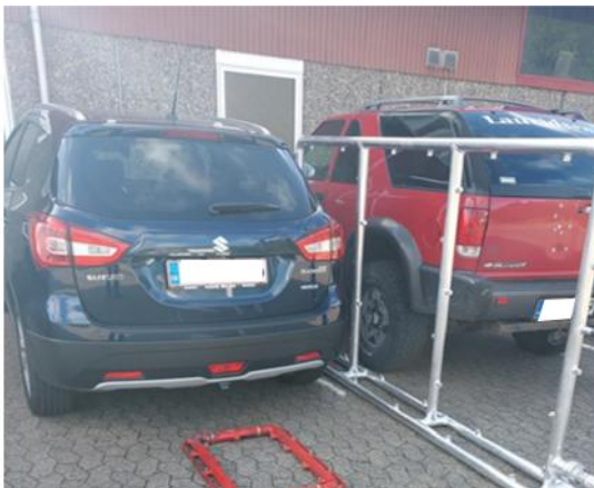
Figure 20 – Specialised sprinkler rack to cool burning EV and avoid spreading.
