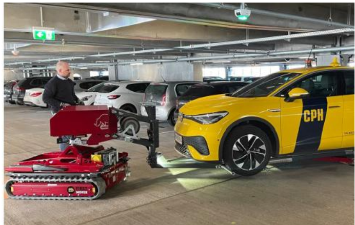
Figure 21 – FirstMover-tool used to move EVs in case of fire.
