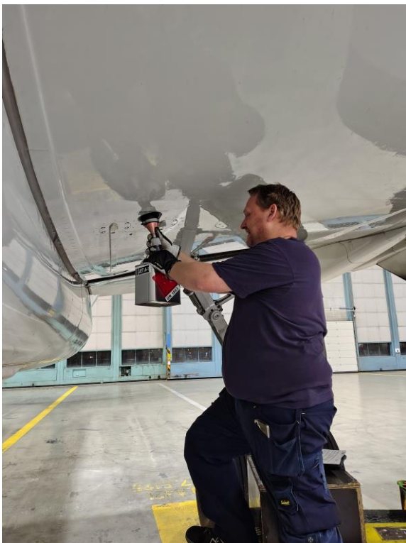
Figure 12: Fuel sampling from the dispenser of DRS during the FuelTrack CPH campaign. (2 of 2)
