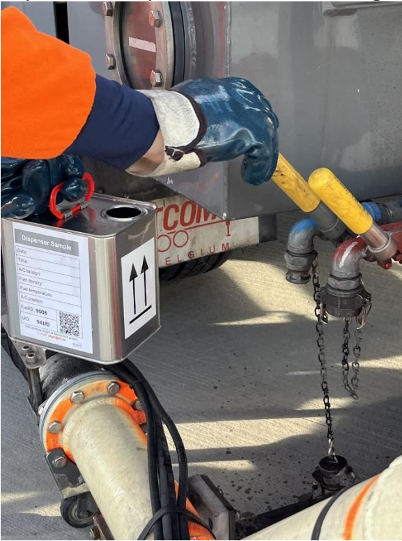
Figure 11: Fuel sampling from the dispenser of DRS during the FuelTrack CPH campaign. (1 of 2)
