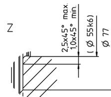
See technical data sheet for available clamping hub diameters (mass moment of inertia). Dimensions available on request.
