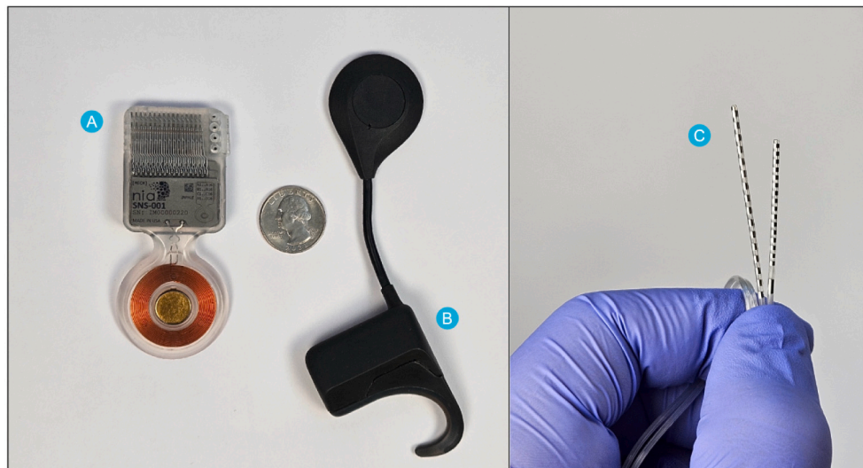
Fig. 2. The Smart Neurostimulation System prototype, including (a) the implantable pulse generator; (b) the external processor; and (c) depth leads containing up to 16 electrodes each. All device materials were selected for biocompatibility and prior medical device usage. The silicone-encapsulated IPG houses a hermetically sealed titanium can surrounding the embedded electronics, platinum/iridium, stainless steel and Pellethane in the lead connector assembly, and Parylene-C surrounding the gold-coated magnet. The depth lead utilizes platinum/iridium electrodes, a stainless-steel set screw block, and a pellethane lead body. EP materials include ABS plastic, nylon and silicone. A U.S. quarter illustrates the scale of the device.
